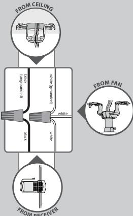
Turn the splices upward and push them carefully back through the hanger bracket into the outlet box. Spread the wires apart, with the grounded wires on one side of the outlet box and the ungrounded wires on the other side of the outlet box.
